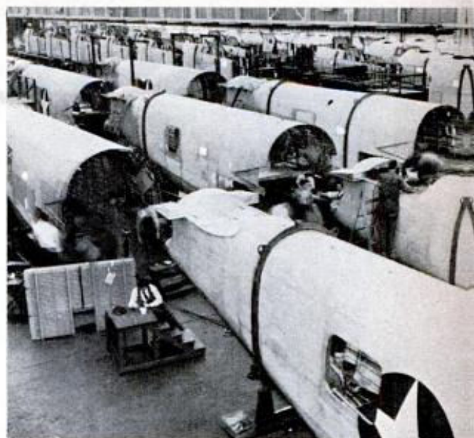
24 Fuselages, each assembled from a dozen parts, take shape in another part of the plant. In the foreground are the aft fuselage sections receiving finishing touches; at rear, forward sections
